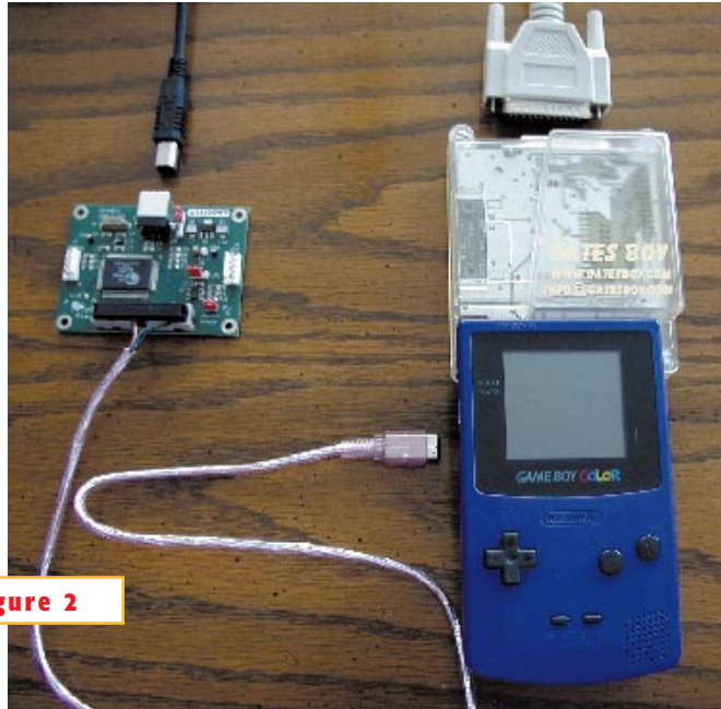
The development system includes a Gameboy Color with a Gatesboy cartridge inserted (right). The parallel cable (top right) allowed program downloading to the flash memory. A modified game-link cable connects the Gameboy to the DevaSys USB I 2 C/I/O interface board (left), and the USB cable (top left) completes the datapath to the desktop computer.
